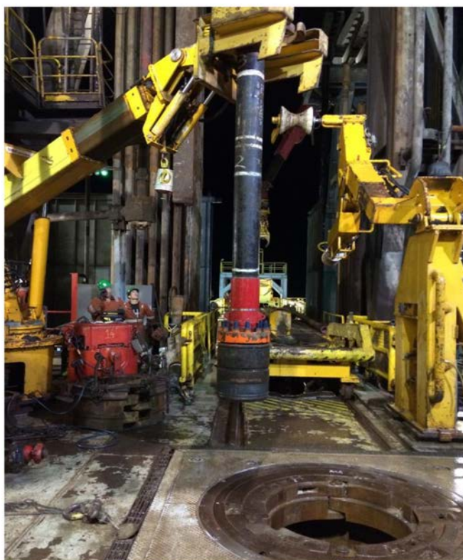
Figure 5—RCD bearing connected to the bottom of the riser.
